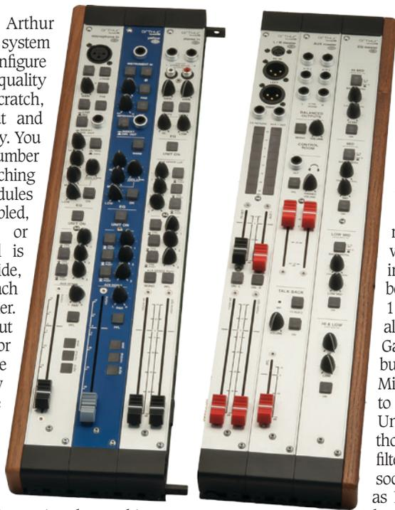
dual status buttons that flip between blue and orange. There is method to the madness, but it is all fairly dazzling! Rotary knobs are domed with clear pointers — these save space and are pleasant to use. Meters use large square LEDs.
